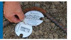
Any bend with an inside diameter less than the diameter of the selected disc, does not comply with New Zealand Standards.
